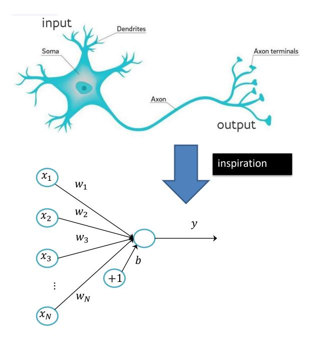
Artificial neural networks (ANN) are an information processing technology inspired by the information processing technique of the human brain. With ANN, the working style of the simple biological nervous system is imitated. Here wi coefficients, xi input values and b gives the tendency or trend parameter. (i=1,2,3, ..., N)
